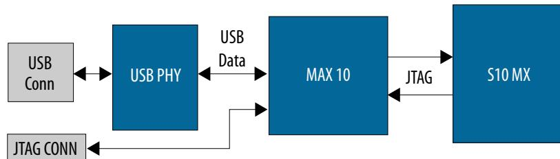
Connection on the external JTAG header (J9) automatically disables the on-board JTAG Intel FPGA Download Cable II. This allows the use of an external USB JTAG dongle to access the JTAG bus on the board.
