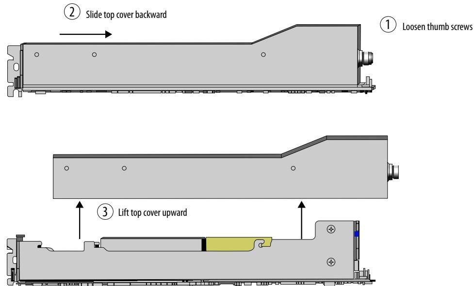
Note: Top cover is required for proper cooling of the board
