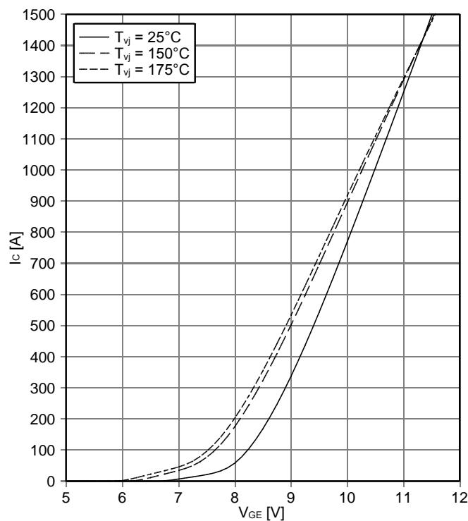
output characteristic IGBT,Inverter (typical)
