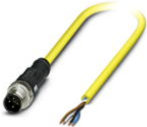
Sensor/Actuator cable, 4-position, PVC, Yellow RAL 1021, Plug straight M12-SPEEDCON, A-coded, on Free cable end, Cable length: 10 m
