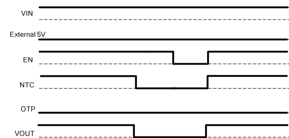
Figure 3: Normal Mode without external 5V → NTC protection Mode → EN Restart
