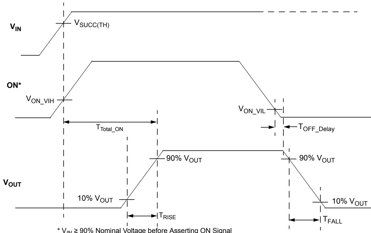
\*  $V_{IN} \geq 90\%$  Nominal Voltage before Asserting ON Signal
