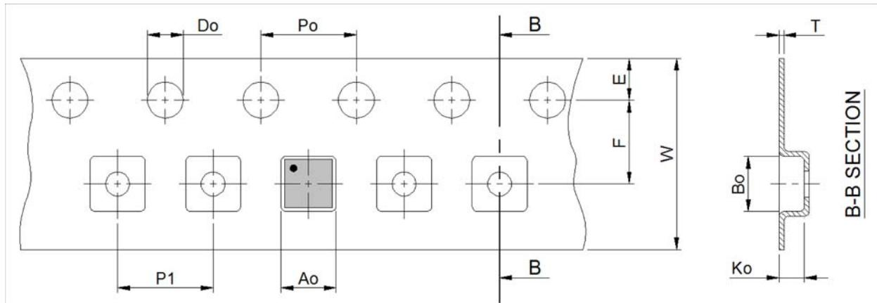
Note: 1. Orientation in carrier: Pin1 is at upper left corner (Quadrant 1).
