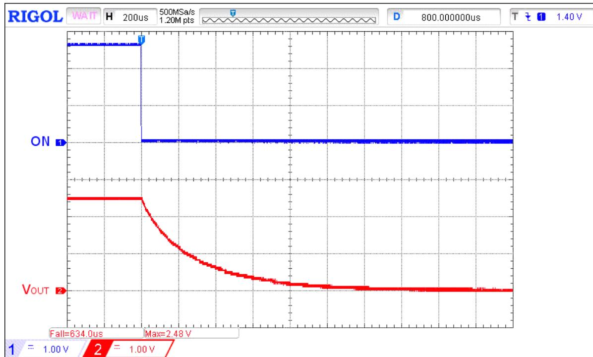
Figure 4. Typical Turn OFF operation waveform for  $V_{IN} = 2.5$  V,  $C_{LOAD} = 30 \mu\text{F}$ ,  $R_{LOAD} = 10 \Omega$
