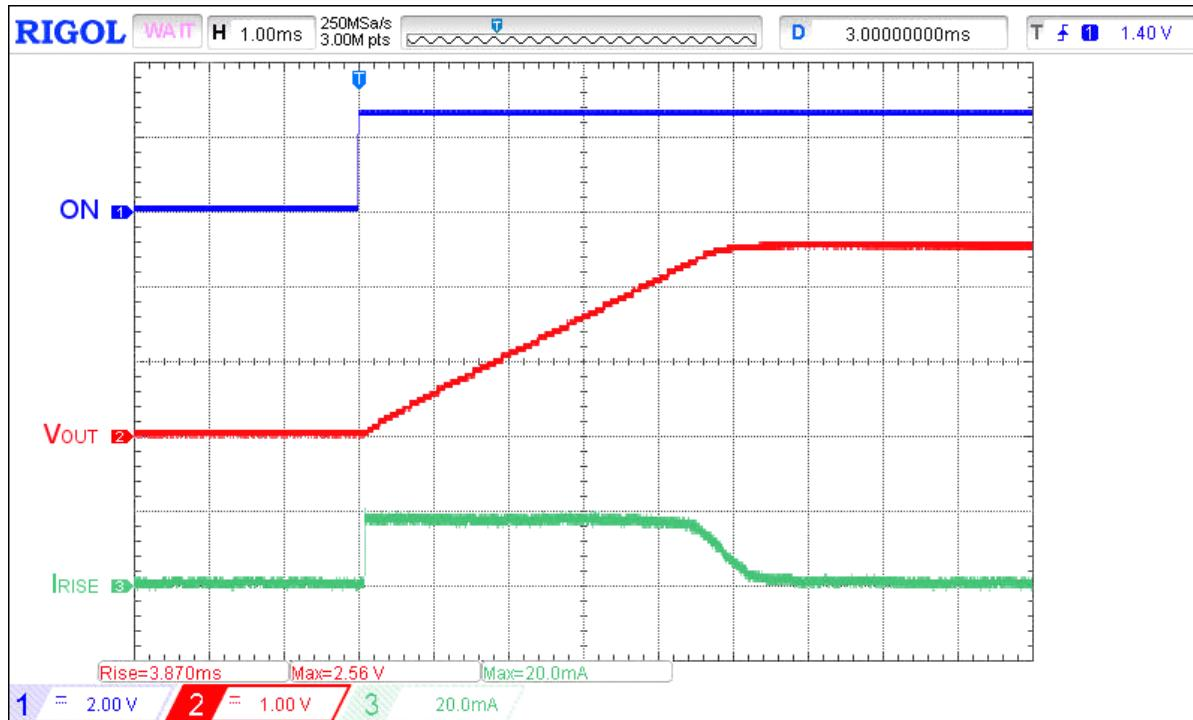
Figure 1. Typical Turn ON operation waveform for  $V_{IN} = 2.5$  V,  $C_{LOAD} = 30 \mu F$
