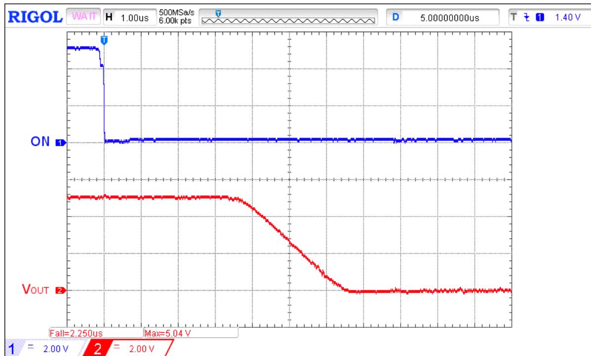
Figure 5. Typical Turn OFF operation waveform for  $V_{IN} = 5$  V, no  $C_{LOAD}$ ,  $R_{LOAD} = 10 \Omega$
