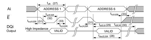
u: W must be HIGH when E is LOW during the address sequence in order to initiate a nonvolatile cycle. G may be either HIGH or LOW throughout. Addresses 1 through 6 are found in the mode selection table. Address 6 determines wheter the U637H256 performs a STORE or RECALL.
