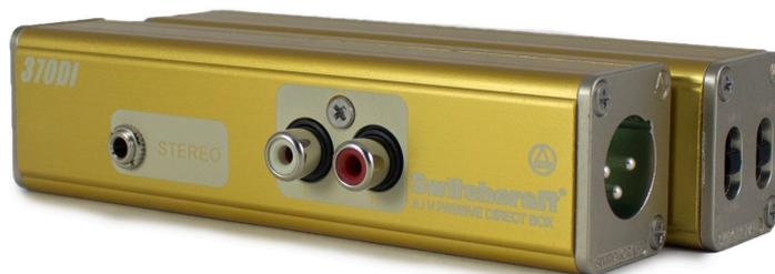
The 370DI is a durable, pocket size, Direct Box which is a cross between Switchcraft's SC700CT DI Box and 318 Inline Audio Adapter. The 370DI sums and converts the unbalanced stereo outputs of cell phones, tablets, laptops and consumer gear to a balanced mono line level for connecting to audio consoles and house sound systems.
