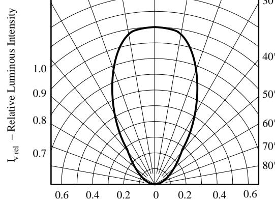
Figure 4 Rel. Luminous Intensity vs. Angular Displacement
