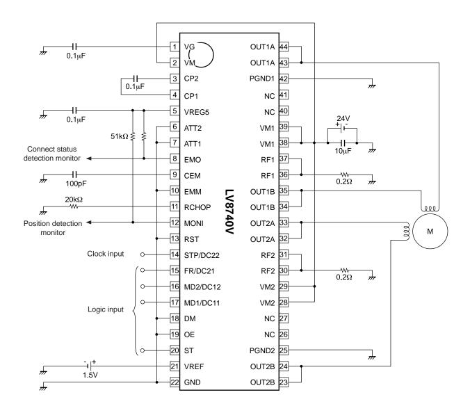
Each constant setting type in the example of the above-mentioned circuit is as follows. When setting current ratio = 100%, VREF = 1.5V, the following output current flows:
