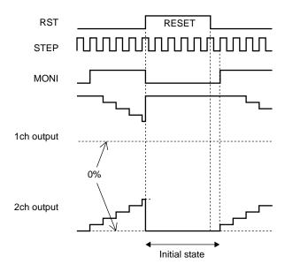
When the RST pin is set High, the output excitation position is forced to the initial state, and the MONI output enters ON a state. When RST is set Low after that, the excitation position proceeds to the next STEP input.
