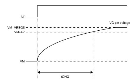
VG Pin Voltage Schematic View
