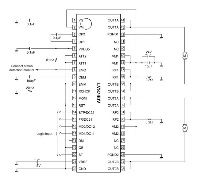
Each constant setting type in the example of the above-mentioned circuit is as follows. When setting current LIMIT = 100%, VREF = 1.5V, the following output current flows:
