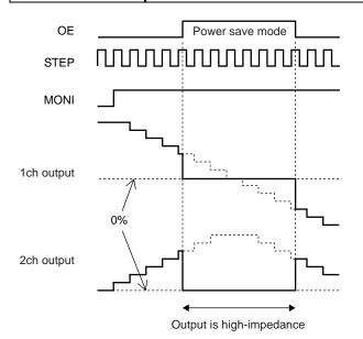
When the OE pin is set High, the output is forced OFF and goes to high impedance.
