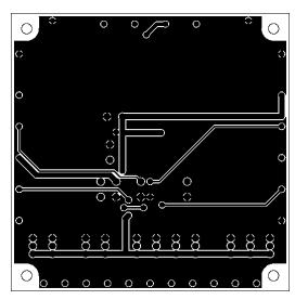
L2: Copper wiring pattern diagram
