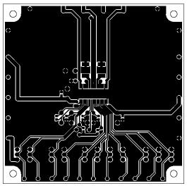
L1: Copper wiring pattern diagram
