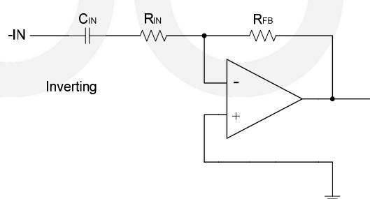
**Figure 2 Differential, Inverting and Non-inverting Gain Configurations**
