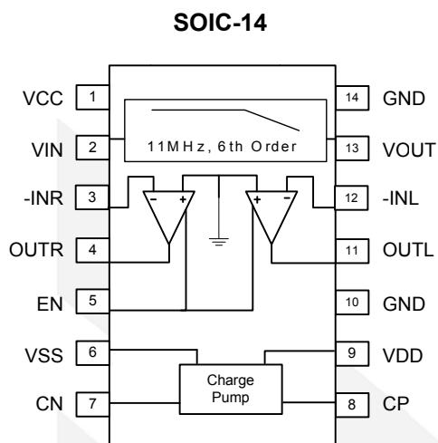
**Figure 1 Pin Assignment**
