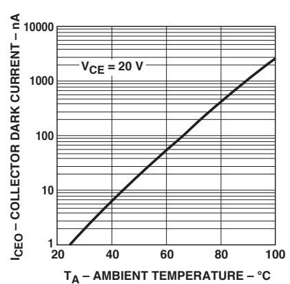
Figure 9. Collector dark current vs. ambient temperature.
