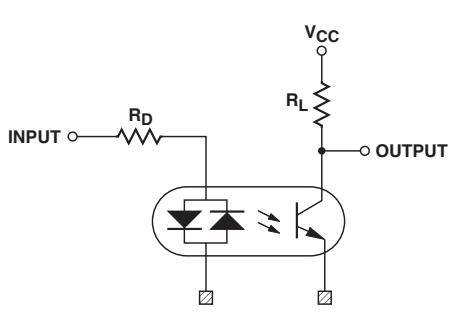
Figure 12. Test circuit for response time.
