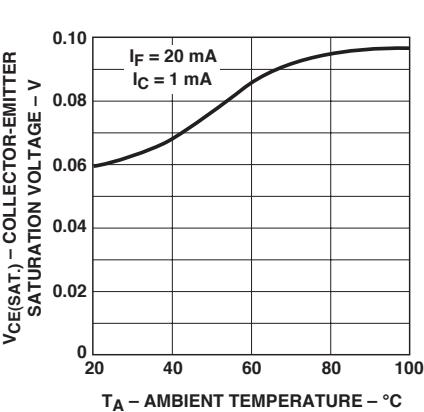
Figure 8. Collector-emitter saturation voltage vs. ambient temperature.
