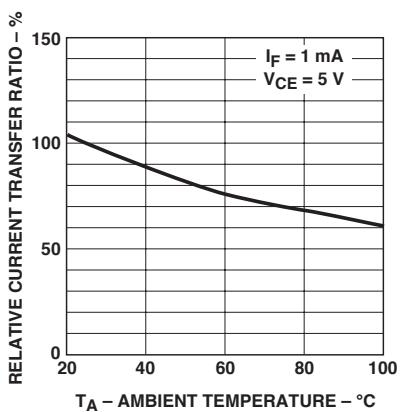
Figure 7. Relative current transfer ratio vs. ambient temperature.
