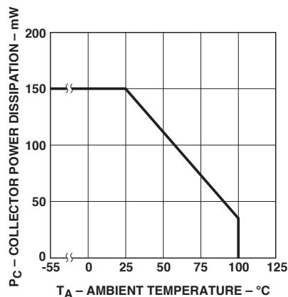
Figure 2. Collector power dissipation vs. ambient temperature.
