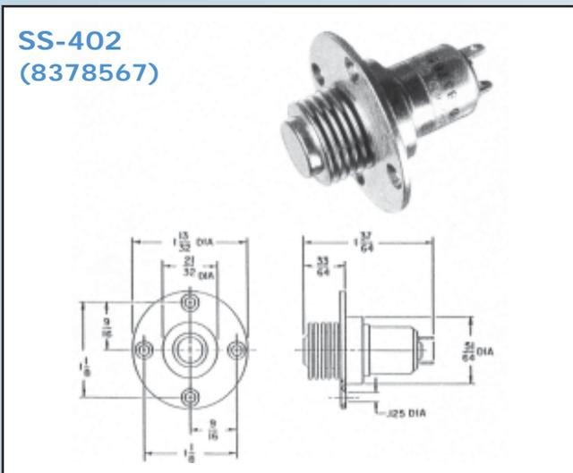
**Push-Button Bellows Switch, Watertight**
