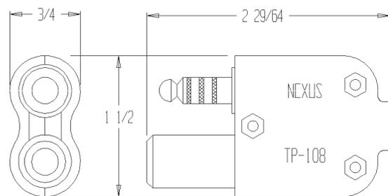
**Telephone Plug Biaxial Shielded
