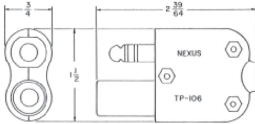
**Telephone Plug Biaxial Shielded
