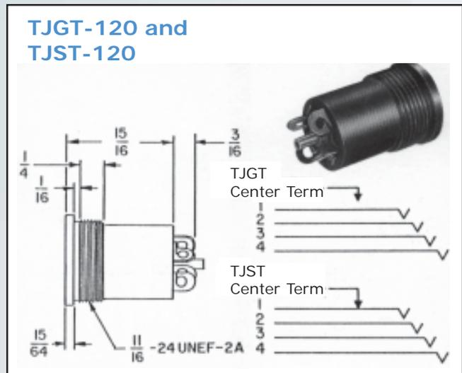
**Threaded Front-Mounted Jack With Switches**
