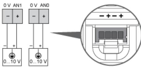
The (-) poles are connected internally.
