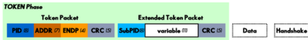
Figure 17 (above) : Extended Token Transaction
