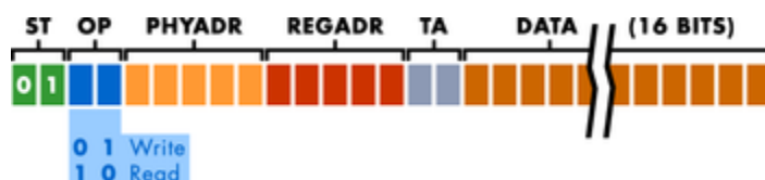
Figure 27 : Basic MDIO Frame Format
