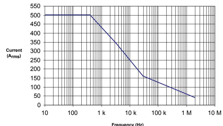
**Maximum Input Current vs. Frequency**
