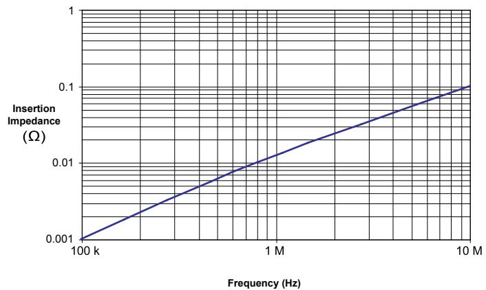
**Insertion Impedance vs. Frequency (typical)**
