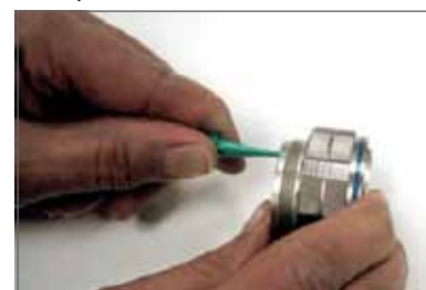
Plastic tool with contact in proper position.
