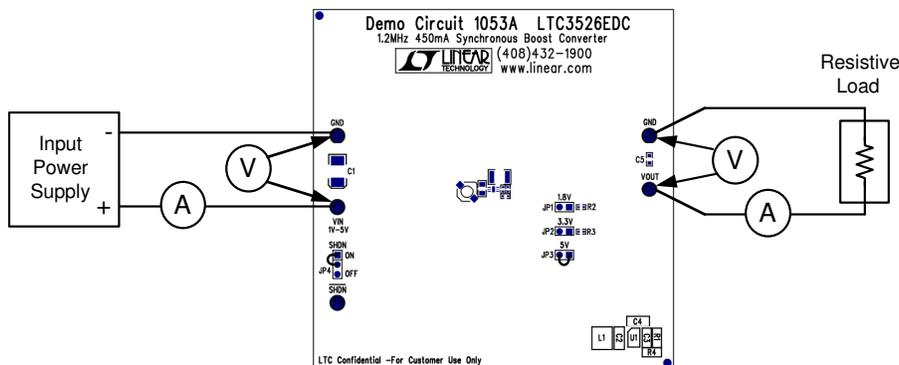
**Figure 1. Demonstration Circuit Test Setup**
