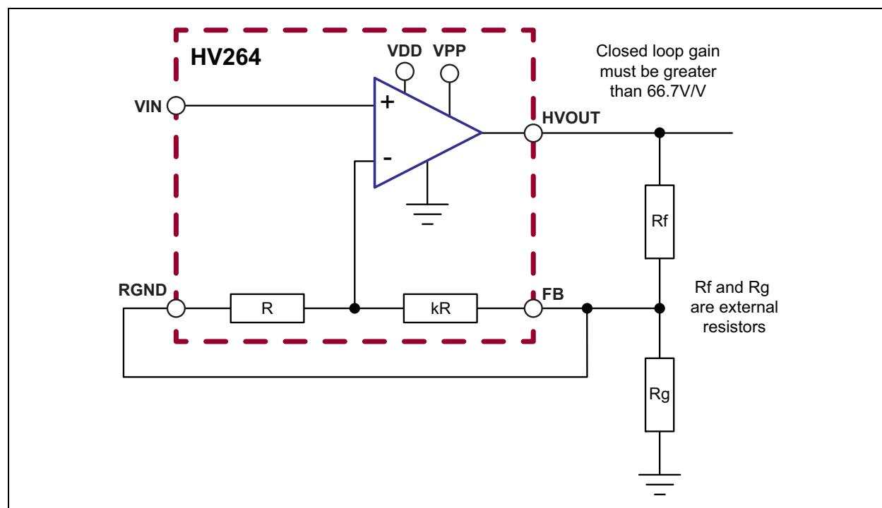
**FIGURE 4-1:** Application Circuit with External Gain Setting Resistors.
