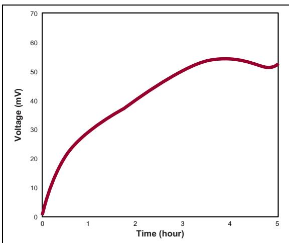
**FIGURE 2-5:** Typical  $HV_{OUT}$  Drift Over Time ( $V_{PP} = 200V$ ,  $V_{DD} = 5.5V$ ,  $V_{IN} = 0.2V$ , Room Temperature and 50 pF Output Loading).
