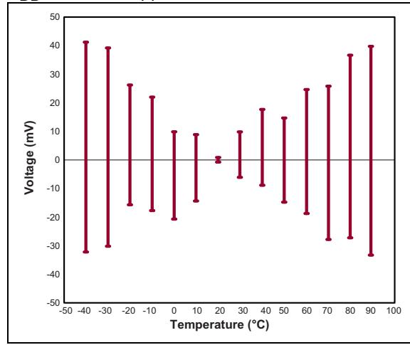
**FIGURE 2-4:** Distribution of Typical  $HV_{OUT}$  Deviation over Temperature ( $V_{IN} = 0.1 V_{DC}$ ,  $1.6 V_{DC}$ ,  $3.3 V_{DC}$ , in reference to  $20^{\circ}C$ ).
