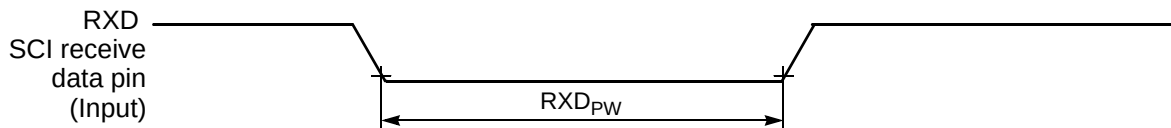
Figure 10-16 RXD Pulse Width
