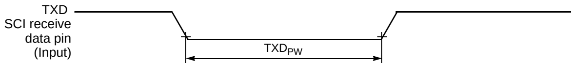
Figure 10-17 TXD Pulse Width
