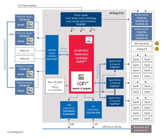
Thanks to its state-of-the-art safety features, the new TriCore<sup>™</sup> AURIX<sup>™</sup> family enables systems to achieve the highest safety level up to ASIL-D. Its scalability allows the selection of a single-core solution for basic airbag systems and multicore solutions for airbag systems with an integrated sensor cluster. The best cost-performance fit is offered by the wide range of flash, performance and peripheral options available within the AURIX<sup>™</sup> family.
