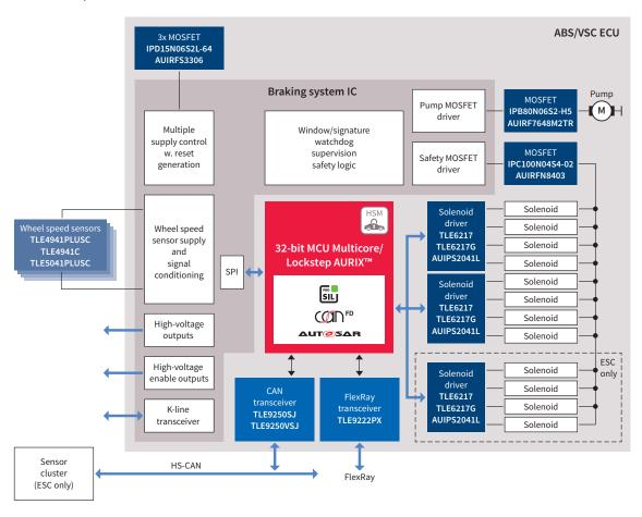
Thanks to its state-of-the-art safety features, the new TriCore<sup>™</sup> AURIX<sup>™</sup> family enables systems to achieve the highest ASIL-D safety level, which is already required in contemporary braking systems. The latest diverse lockstep technology with clock delay (diverse lockstep core) significantly reduces the software overhead and enables fast time-to-market. The scalability supports an optimized cost-performance fit for basic ABS systems up to highly integrated ESC systems.
