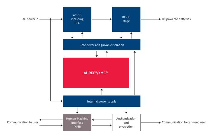
Off-board charging, where users can charge plug-in hybrids and pure EVs in private garages and open parking lots, demands an optimized solution with high MCU switching frequency to stay efficient and cost competitive. The Infineon XMC™ family is the answer! If you have security or safety requirements, you can scale from XMC™ family to AURIX™ to support your solution.
