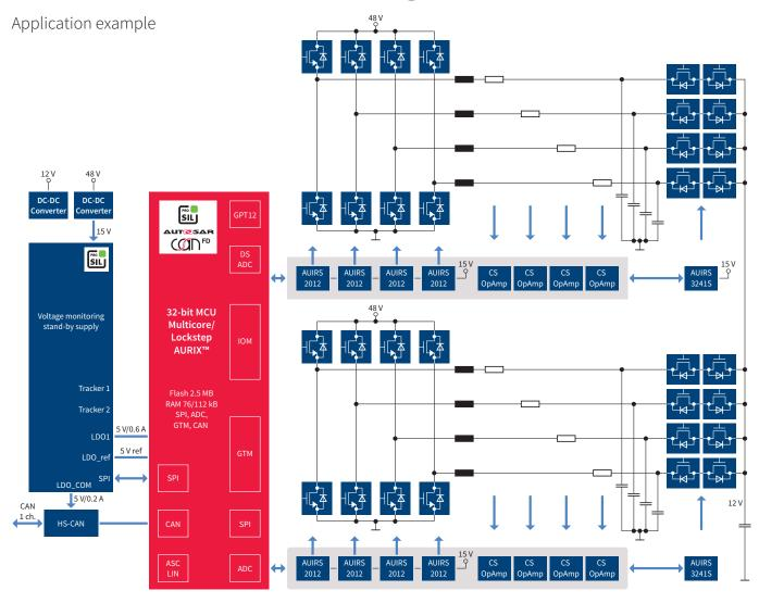
The DC-DC converter ECU is responsible for the conversion of voltage between the low voltage domain (typically 48 V to 60 V) and the 12 V domain in mild hybrid cars. The 48 V domain powers stop-start motors, hybrid motors, and turbochargers, enabling engine downsizing and better fuel economy and performance.
