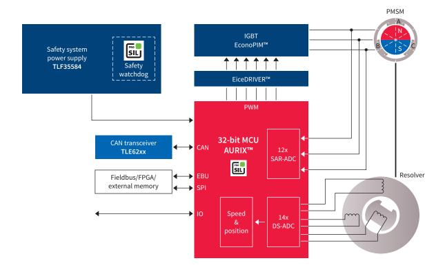
Inverters are key components and, regardless of whether the motor is synchronous, asynchronous or brushless DC, the inverter always functions in a similar way and is controlled by an integrated PCB, which should be designed to minimize switching losses and maximize thermal efficiency. Infine on is providing you solutions to support those requirements.s
