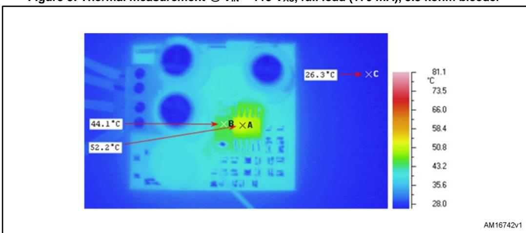
**Figure 6: Thermal measurement @  $V_{IN} = 230$  V<sub>AC</sub>, full load (170 mA), 3.3 kohm bleeder**
