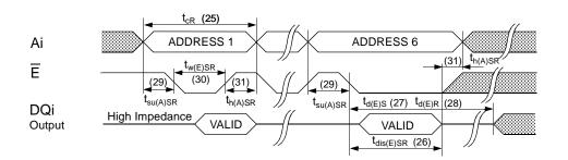
t: W must be HIGH when E is LOW during the address sequence in order to initiate a nonvolatile cycle. G may be either HIGH or LOW throughout. Addresses 1 through 6 are found in the mode selection table. Address 6 determines whether the U631H16 performs a STORE or RECALL.
