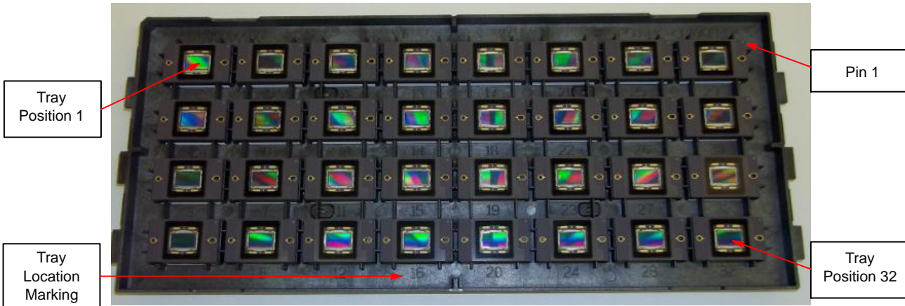
Figure 38. Tray Pin-Down View
