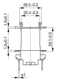
Hole arrangement View in mounting direction
