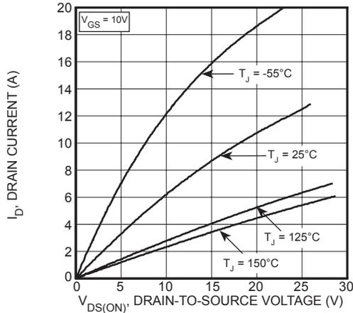
Figure 1, Output Characteristics
