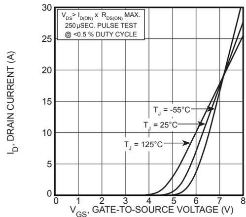
Figure 4, Transfer Characteristics
