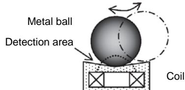
\*4. Whether the metal ball built in the sensor is detected or not determines the ON/OFF state of the output transistor. (Intermittent output)
