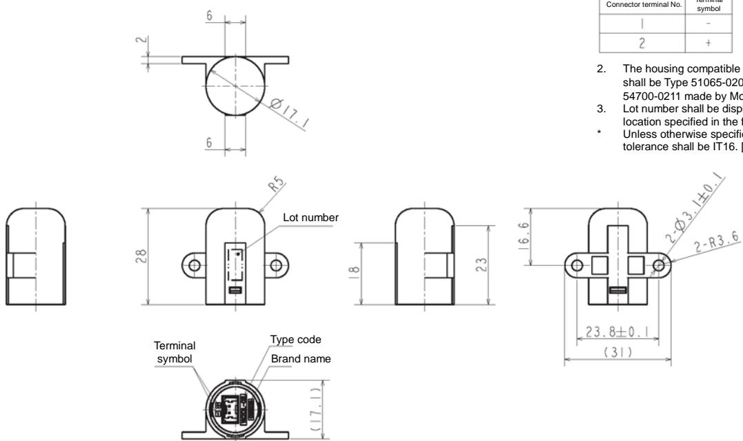
Note: 1. The following shows the relationship between the connector terminal numbers and terminal symbols.
