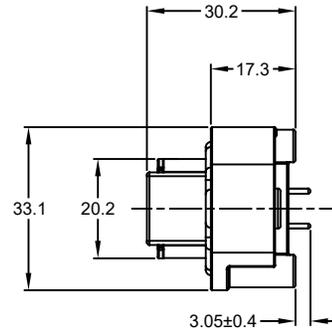
RECOMMENDED SCREW: 4-20 [M3.12 x 1.27] THREAD-FORMING SCREW, TORQUE: 6-10 IN-LB [0.68-1.13 NM]
