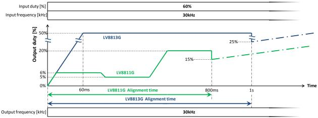
Figure 33. Timing chart example: Alignment duty cycle
