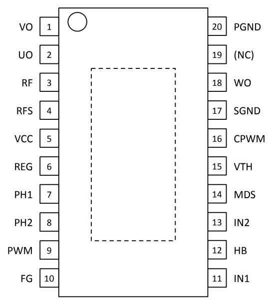
Figure 5. LV8811G, LV8813G Pin Assignment
