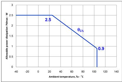
Figure 6. Power Dissipation vs Ambient Temperature Characteristic
