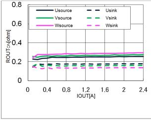
Figure 9. Output ON resistance vs Output current
