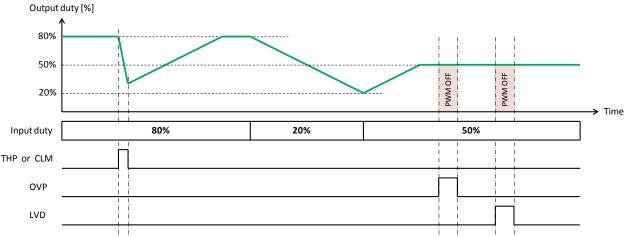
Figure 39. Timing chart example: Protections
