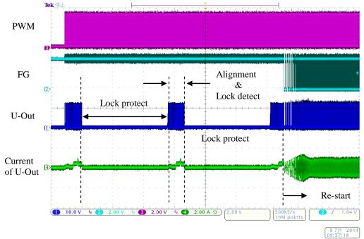
Figure 45. Lock Protection (Case of the LV8811G)
