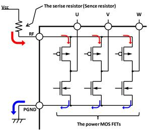
Figure 23. Schematic view of power current route
