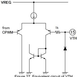
Figure 27. Equivalent circuit of VTH
