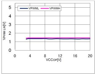
Figure 15. PWM threshold voltage vs VCC voltage
