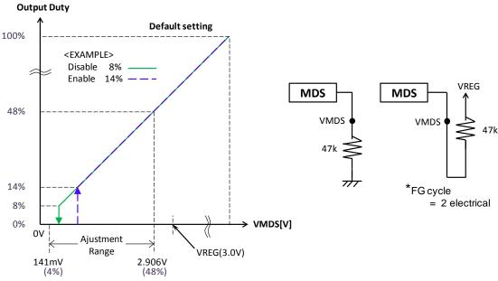
Figure 49. Example Setting Minimum PWM duty cycle (case of default setting)
