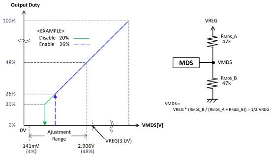
Figure 50. Example Setting Minimum PWM duty cycle (case of 1/2 V<sub>REG</sub> setting)
