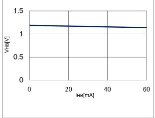
Figure 14. V<sub>HB</sub> output voltage vs HB load current
