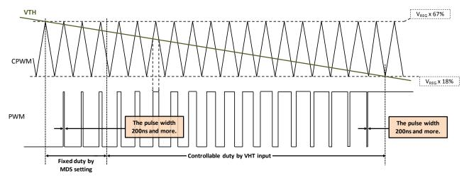
Figure 46. PWM Duty cycle control by CPWM and the VTH voltage
