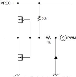
Figure 25. Equivalent circuit of PWM
