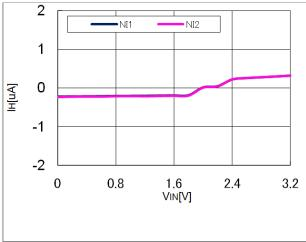
Figure 17. IN1/IN2 input current vs IN1/IN2 input voltage
