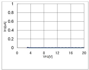
Figure 13. FG leakage current vs FG input voltage
