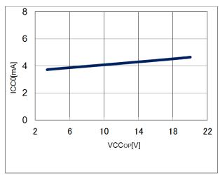
Figure 7. Supply current vs VCC voltage
