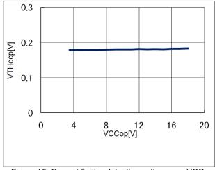
Figure 10. Current limiter detection voltage vs VCC voltage
