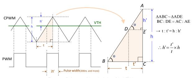
Figure 47. Reference of the calculation of the VTH input range
