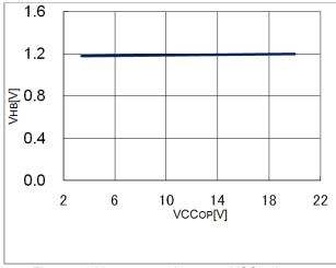
Figure 16. V<sub>HB</sub> output voltage vs VCC voltage
