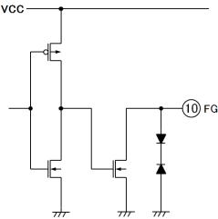
Figure 20. Equivalent circuit of FG
