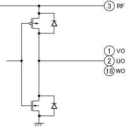
Figure 21. Equivalent circuit of U/V/W
