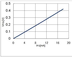
Figure 12. FG output voltage vs FG input current
