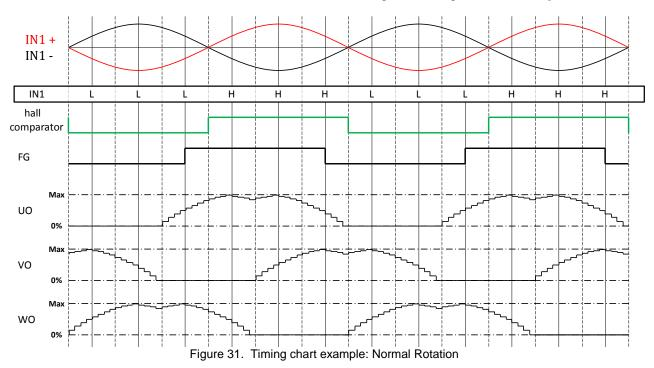
The amplitude of current waveform is effectived by input PWM duty cycle while the sinusoidal waveform is kept.
