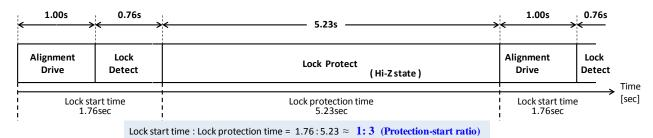
Figure 44. Timing chart example: Lock Protection for LV8813G
