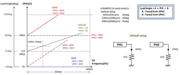
Figure 51. Example Setting Lead Angle (case of default setting)
