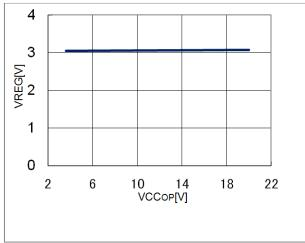
Figure 8. V<sub>REG</sub> output voltage vs VCC voltage
