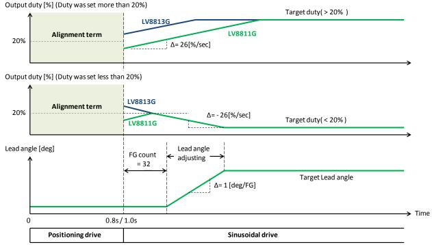
Figure 34. Timing chart example: Positioning and Soft start
