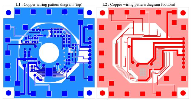
Figure 55. Pattern Diagram of Top and Bottom Layer
