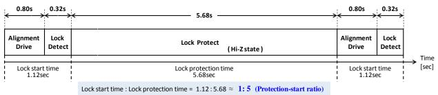
Figure 43. Timing chart example: Lock Protection for LV8811G
