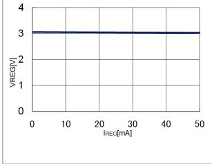
Figure 11. V<sub>REG</sub> output voltage vs REG load current
