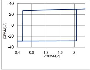
Figure 18. CPWM charge/discharge current
