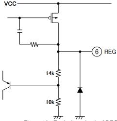
Figure 19. Equivalent circuit of REG
