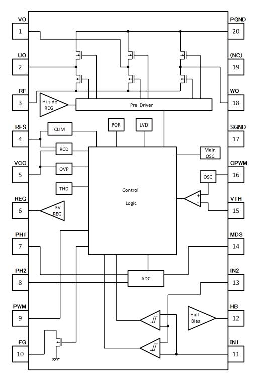
Figure 1. LV8811G, LV8813G Block Diagram
