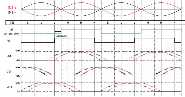
Figure 53. Timing chart example: Lead Angle
