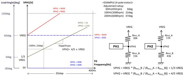
Figure 52. Example Setting Lead Angle (case of 1/3V<sub>REG</sub> and 4/5V<sub>REG</sub> setting)
