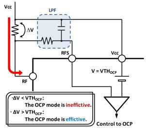
Figure 24. Schematic view of the CLM circuit
