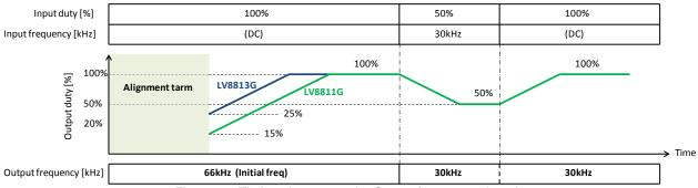
Figure 38. Timing chart example: Output frequency changing
