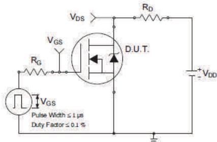
**Fig 20a.** Switching Time Test Circuit
