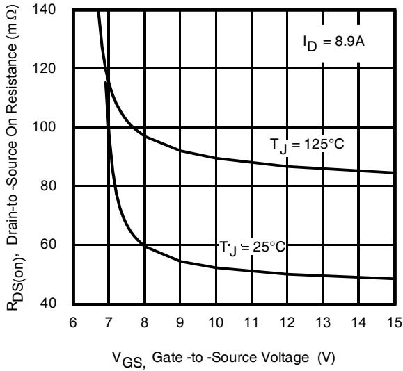
**Fig. 3** Typical On-Resistance vs. Gate Voltage
