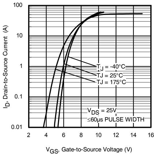
**Fig. 5.** Transfer Characteristics
