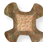
Indenter Crimp Cross-Section Across Axis
