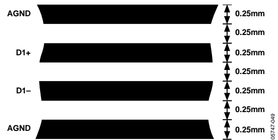
Figure 61. Arrangement of Signal Tracks
