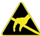
PESW-*-11Y Warning of Static Sensitive Device
