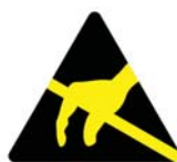
PESW-AA-11Y Warning of Static Sensitive Device
