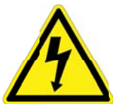
PESW-*-1Y Caution – Risk of Electric Shock
