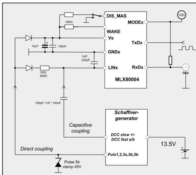
Figure 13: Test circuitry for automotive transients
