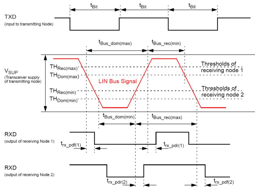
Figure 4: LIN timing diagram (reference LIN2.1 specification)
