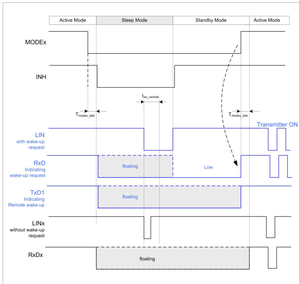
Figure 6: remote wake up and wake-up source recognition
