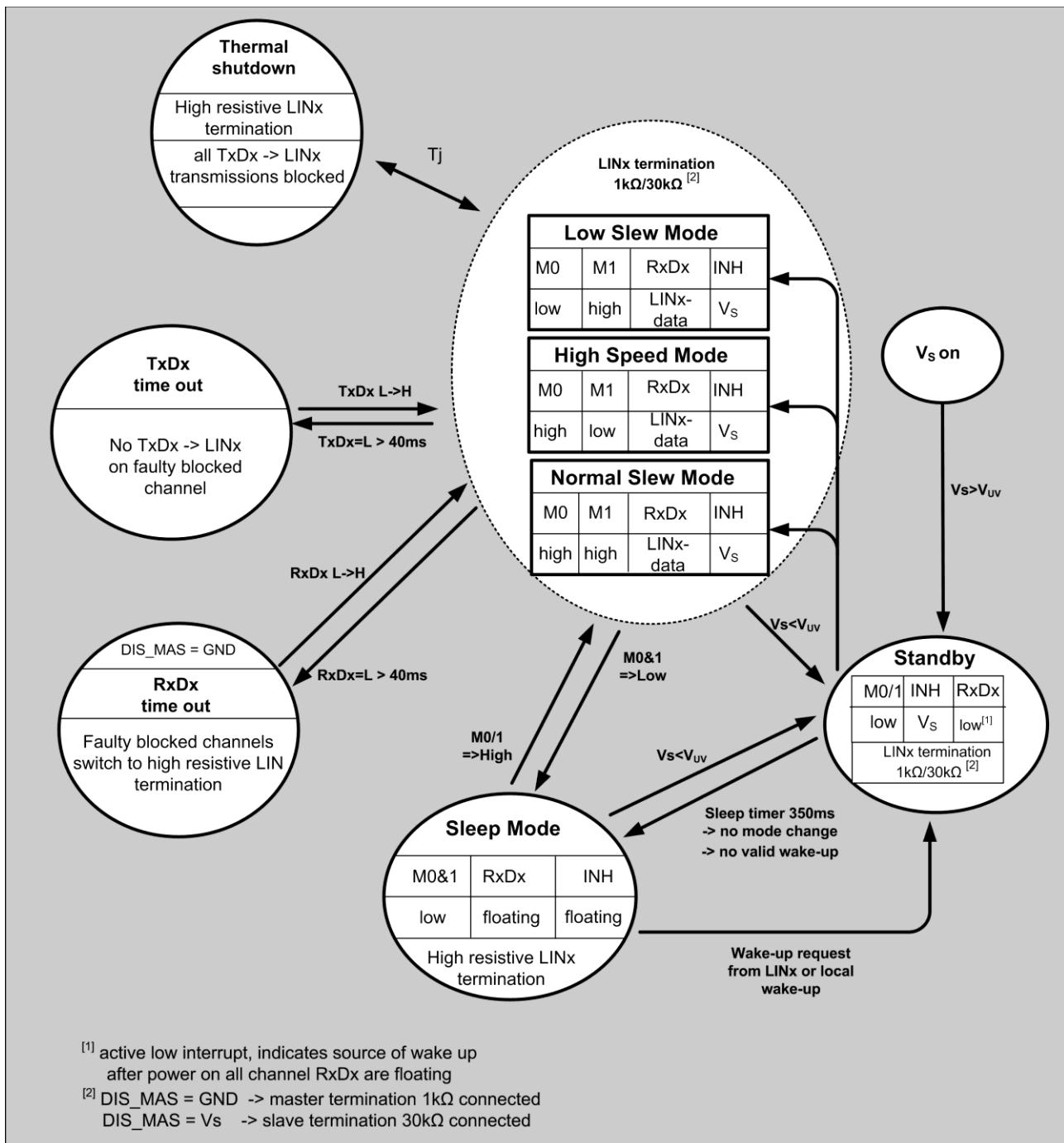
*Figure 5: State Diagram of the MLX80004/2*
