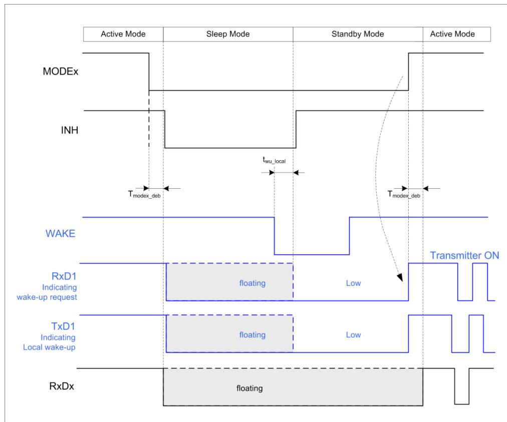
Figure 7: local wake up and wake-up source recognition
