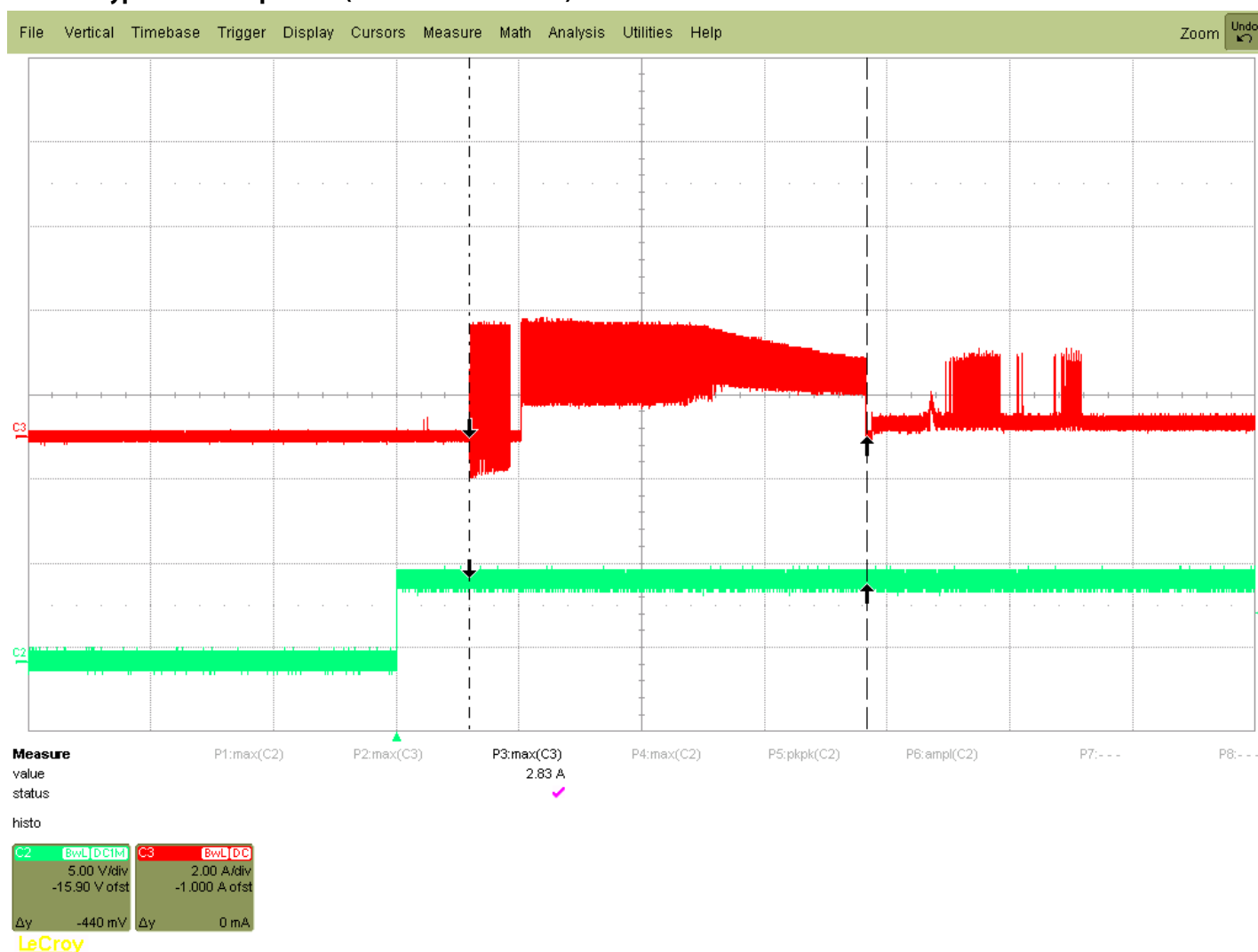
Figure 1. Typical 5V & 12V startup and operation current profile (2TB and 1TB models)
