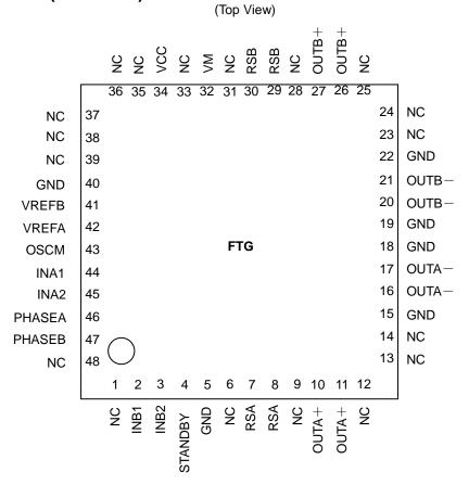
Please mount the four corner pins of the QFN package and the exposed pad to the GND area of the PCB.
