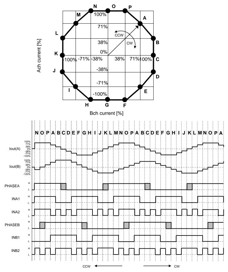
Timing charts may be simplified for explanatory purpose. Please set INA1, INA2, INB1, and INB2 to Low until VM power supply reaches the proper operating range.
