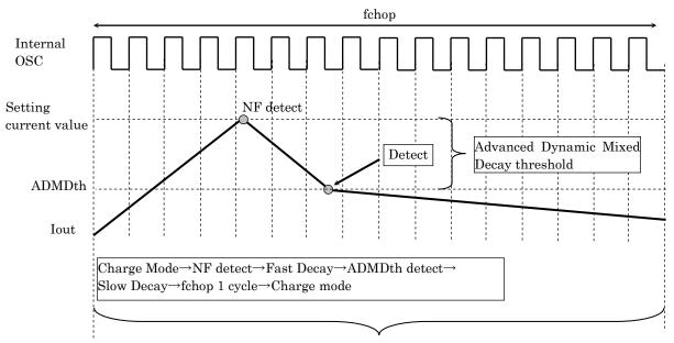
The Advanced Dynamic Mixed Decay threshold, which determines the current ripple level during current feedback control, is a unique value.
