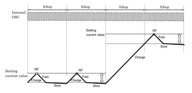
When the Charge period is longer than fchop cycle, the Charge period will be extended until the motor current reaches the NF threshold. Once the current reaches the next current step, then the sequence will go on to ADMD control.
