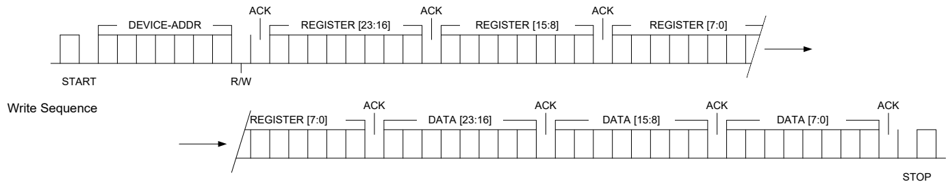
FIGURE 9. I 2 C WRITE SEQUENCE OPERATION
