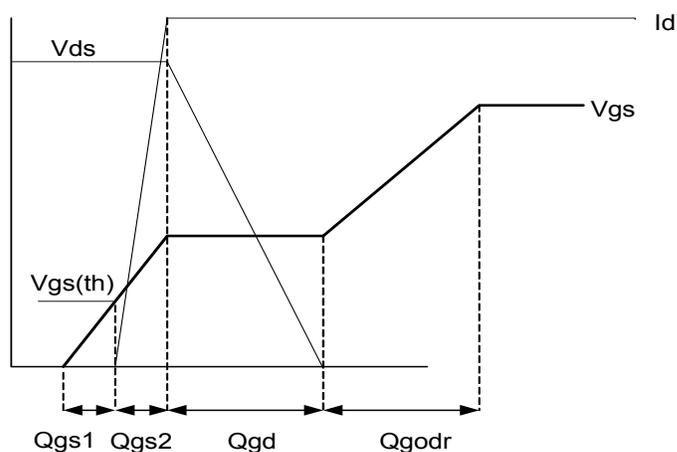
**Fig 13b. Gate Charge Waveform**
