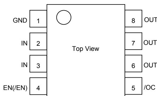
Fig.40 Pin configuration
