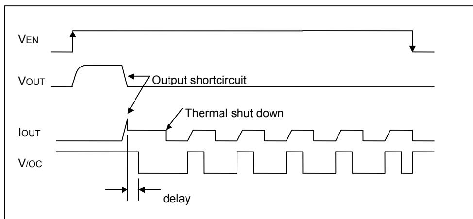
Fig.42 Over-current detection, thermal shutdown timing
