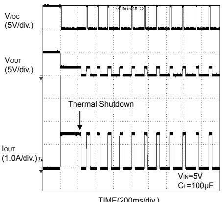
Fig.36 Thermal shutdown
