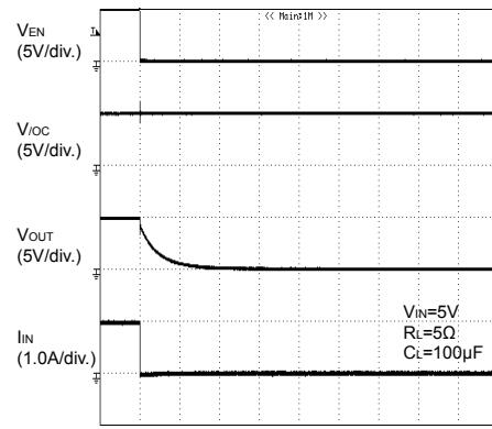
Fig.30 Output fall characteristic
