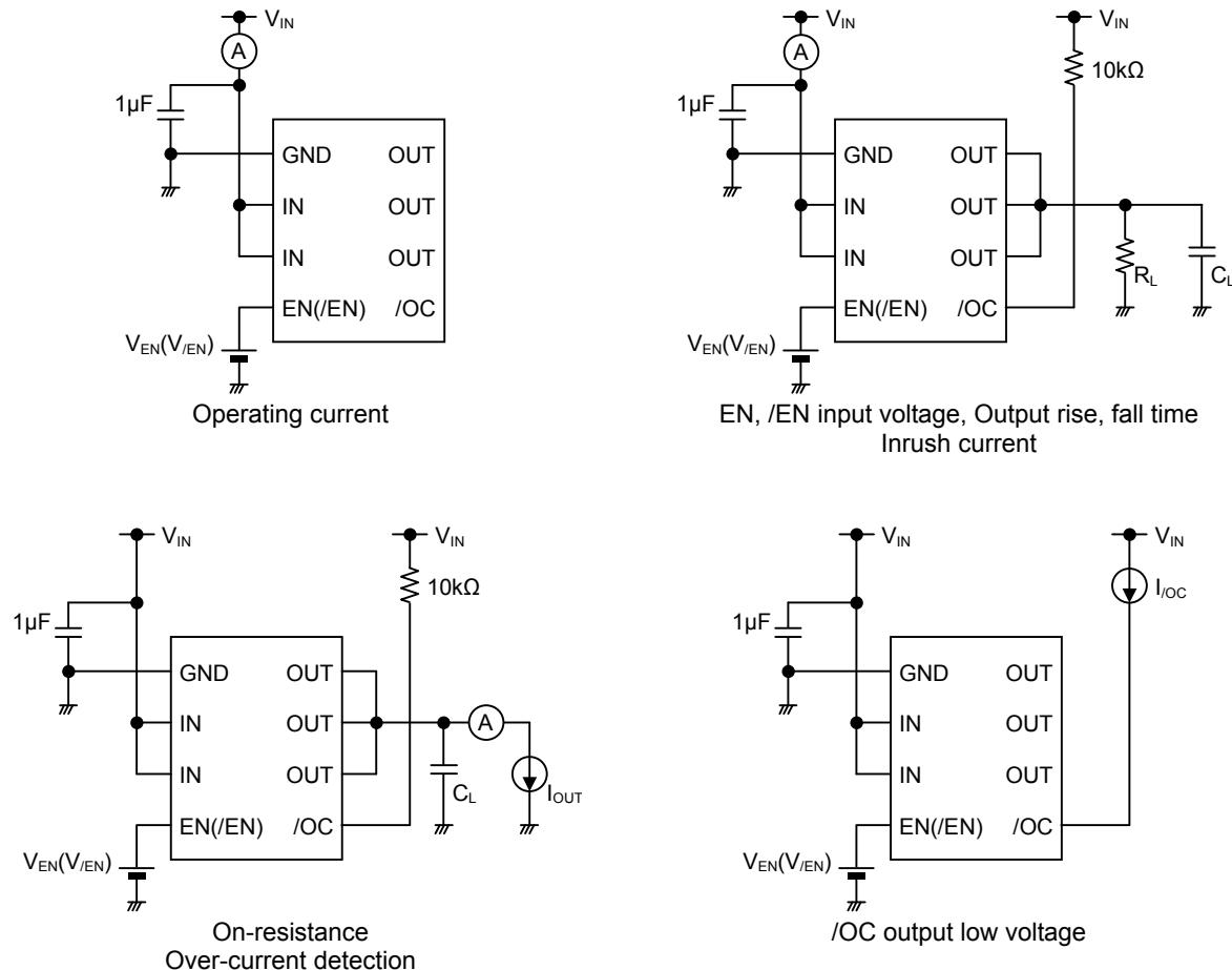
Fig.1 Measurement circuit
