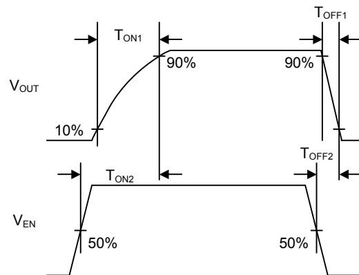
Fig.2 Timing diagram
