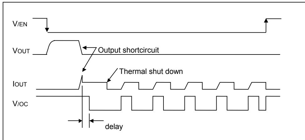
Fig.41 Over-current detection, thermal shutdown timing
