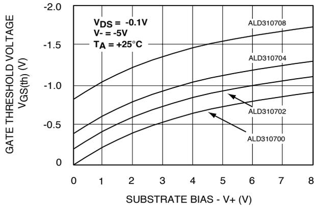
**GATE THRESHOLD VOLTAGE vs. V- VOLTAGE**
