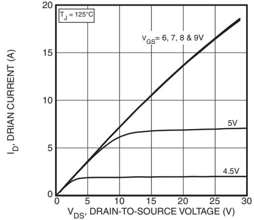
Figure 2, Output Characteristics
