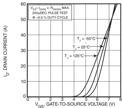
Figure 4, Transfer Characteristics
