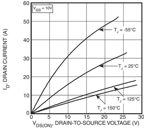
Figure 1, Output Characteristics
