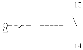
13 Keylock switch 2 positions page 8
