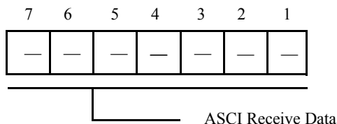
Figure 31. ASCII Receive Register Channel 1R
