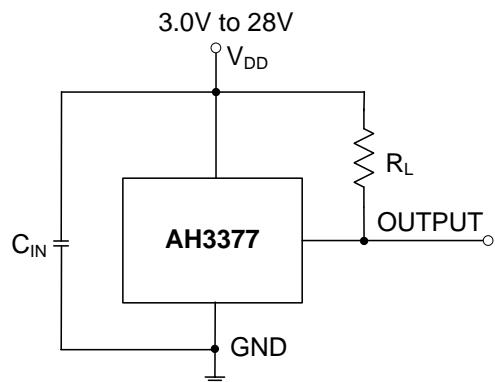
Note: 4. C<sub>IN</sub> is for power stabilization and to strengthen the noise immunity, the recommended capacitance is 10nF ~ 100nF.
