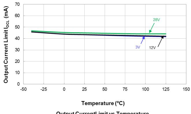
**Temperature (°C)****Output Current Limit vs Temperature**
