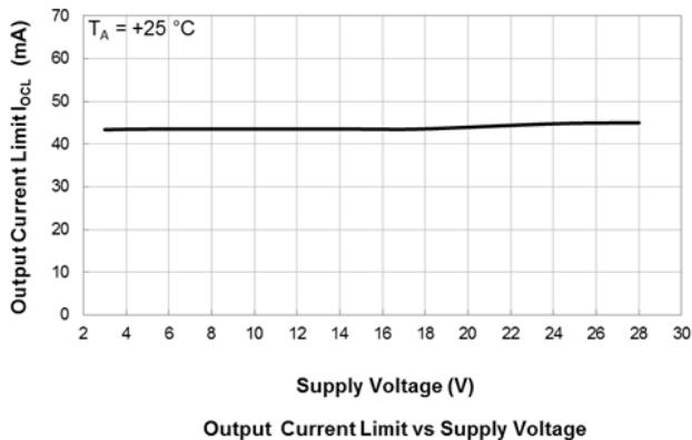
**Supply Voltage (V)****Output Current Limit vs Supply Voltage**
