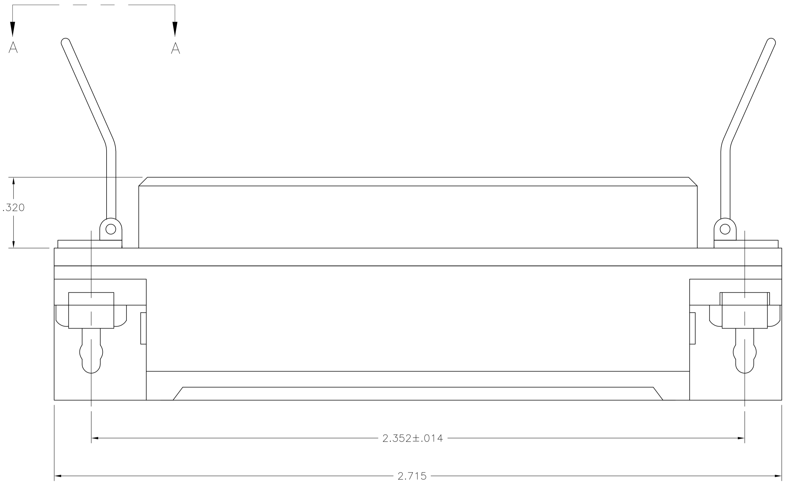
SUGGESTED PRINTED CIRCUIT BOARD MOUNTING DIMENSIONS
