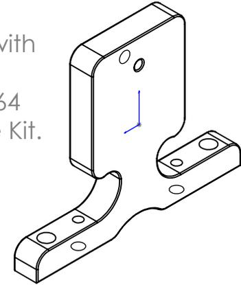
Use the 1/4" #4-40 screws with inner threaded holes, spaced for servo horns.
