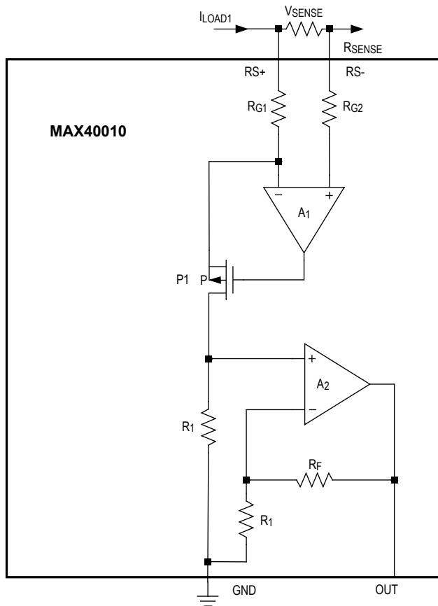
Figure 1 : MAX40010 Functional Diagram
