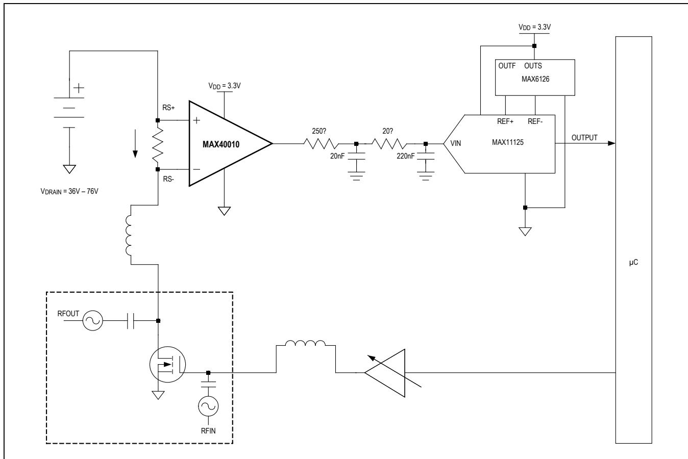
Figure 2: MAX40010 Used in Base Station Application
