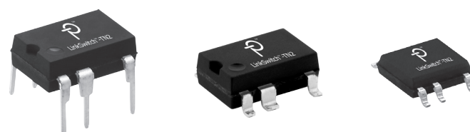
Figure 2. Package Options. P: PDIP-8C, G: SMD-8C, D: SO-8C.
