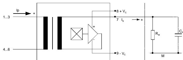
**Possibilities of wiring for  $V_C = \pm 15V$  (@  $T_A = 85^\circ C$ ,  $R_M = 22 \Omega$ )**
