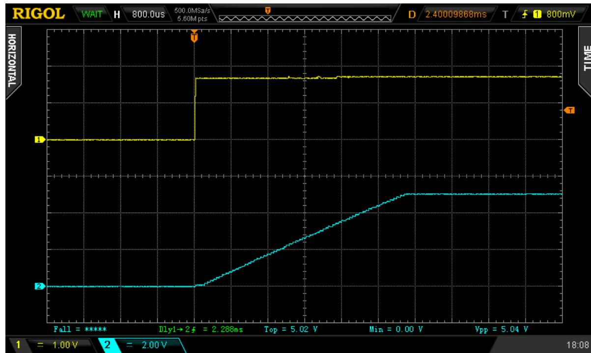
Figure 2. Typical Turn ON operation waveform for  $V_{DD} = V_D = 5 \text{ V}$ ,  $C_{SENSE} = 12 \text{ nF}$ ,  $C_{LOAD} = 10 \mu\text{F}$ ,  $R_{LOAD} = 20 \Omega$
