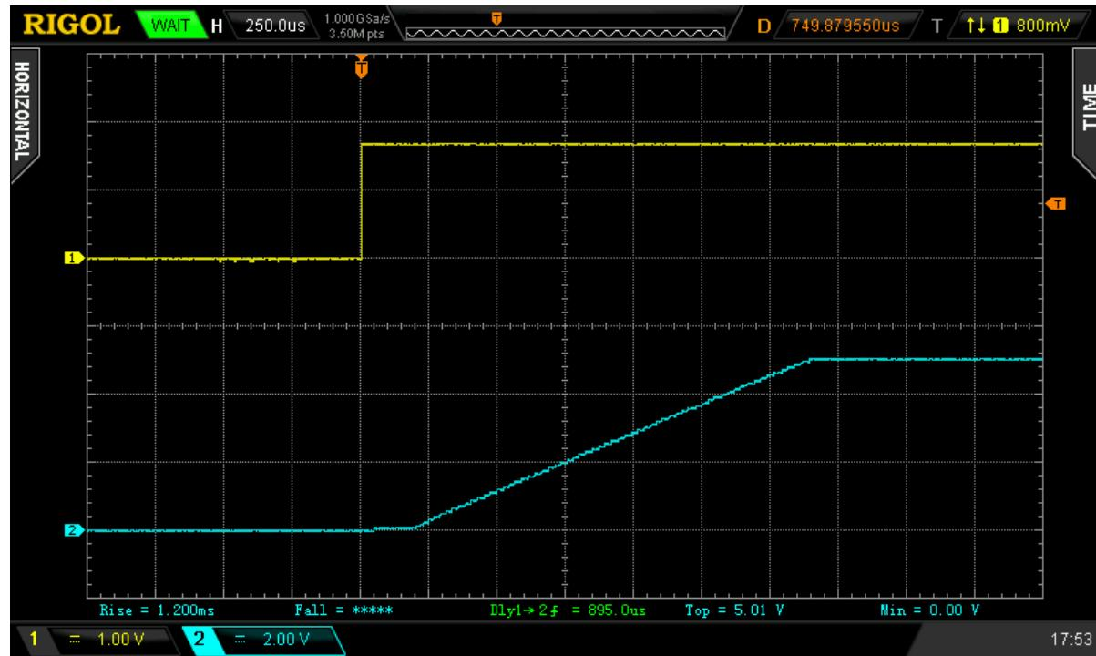
Figure 1. Typical Turn ON operation waveform for  $V_{DD} = V_D = 5 \text{ V}$ ,  $C_{SENSE} = 4 \text{ nF}$ ,  $C_{LOAD} = 10 \mu\text{F}$ ,  $R_{LOAD} = 20 \Omega$
