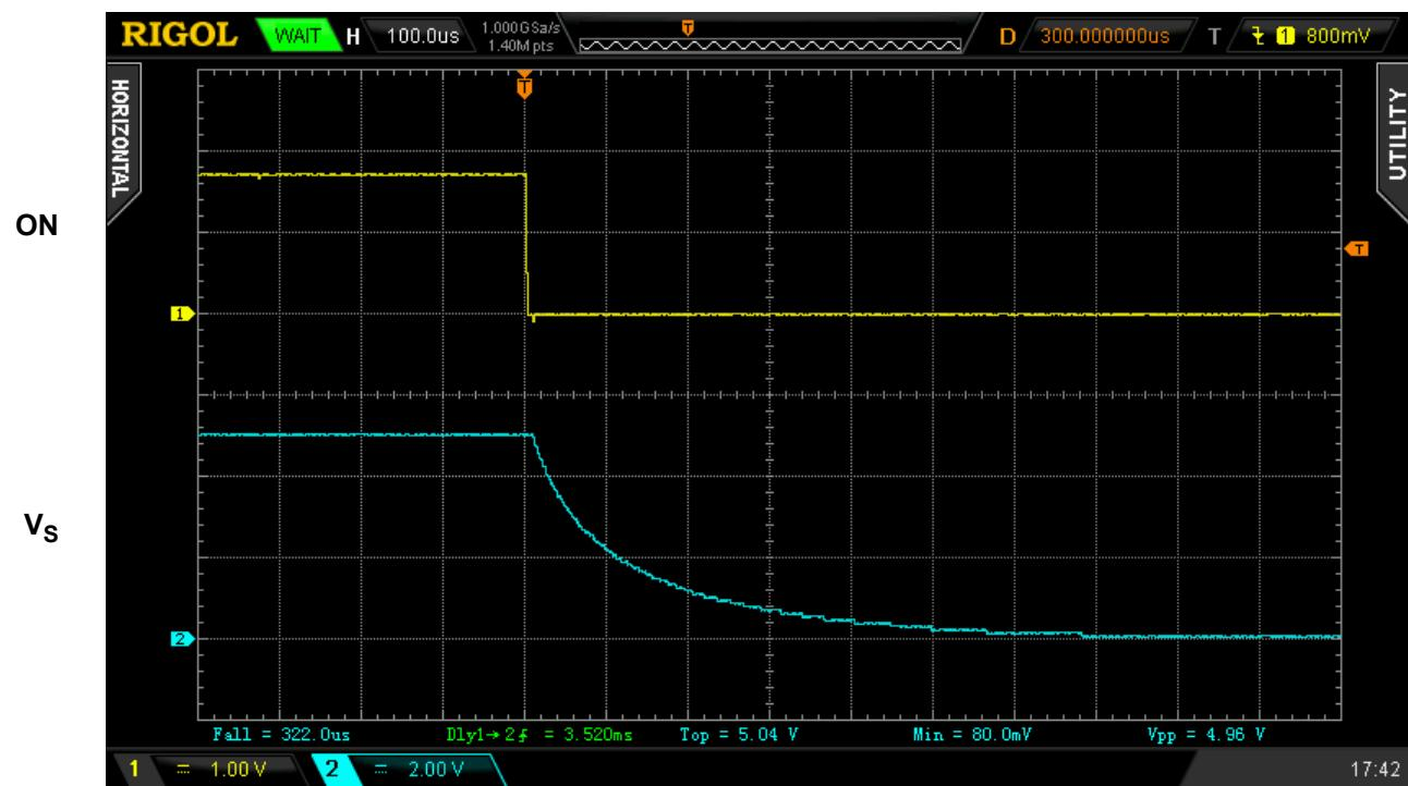
Figure 4. Typical Turn OFF operation waveform for  $V_{DD} = V_D = 5$  V,  $C_{SLEW} = 4$  nF,  $C_{LOAD} = 10 \mu\text{F}$ ,  $R_{LOAD} = 20 \Omega$
